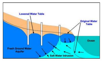
The fresh water floats on top of the salt water. As the fresh water is removed and the hydrostatic pressure it creates is decreased, the salt water come farther into the aquifer Source: http://www.awqinc.com/salt.html
